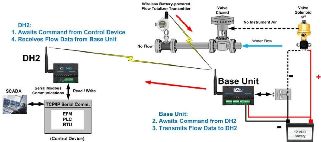
Figure 4 depicts a wireless failsafe closed loop. This wireless application will ensure failsafe protection if the DH2, Control Device or Base Unit electronics fail or loses power. The method behind this application is that all three computer based devices remain in constant communication. This is accomplished using serial Modbus communications between the Control Device and DH2 utilizing the pulsed output function of the Base Unit connected to the valve solenoid equipment.
