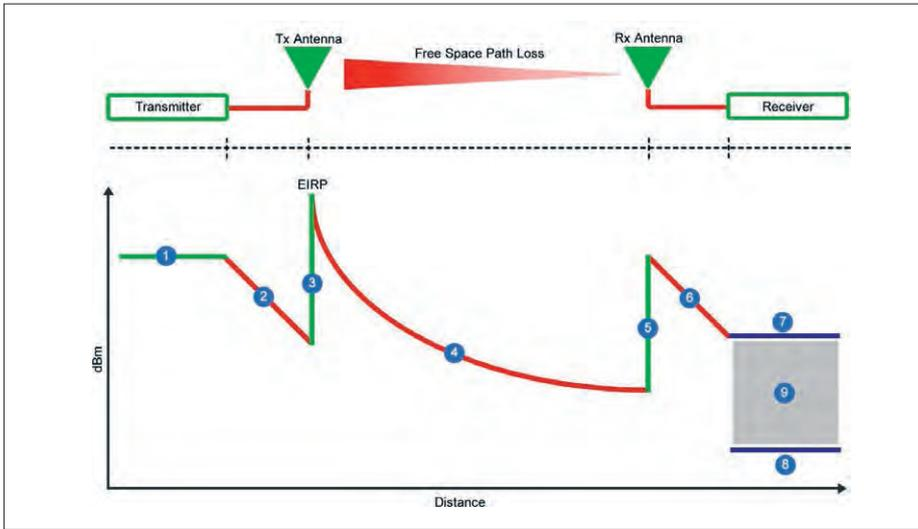
Figure 3: Link Budget. The numbers in this figure correspond with the steps listed in the “Practical Application” section of this article.
