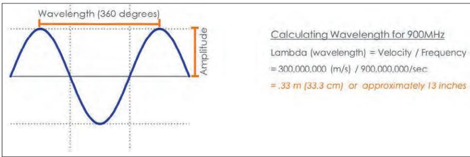
Figure 2: Wavelength and Amplitude
