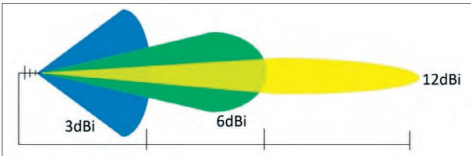
Figure 4: Antenna Gain
