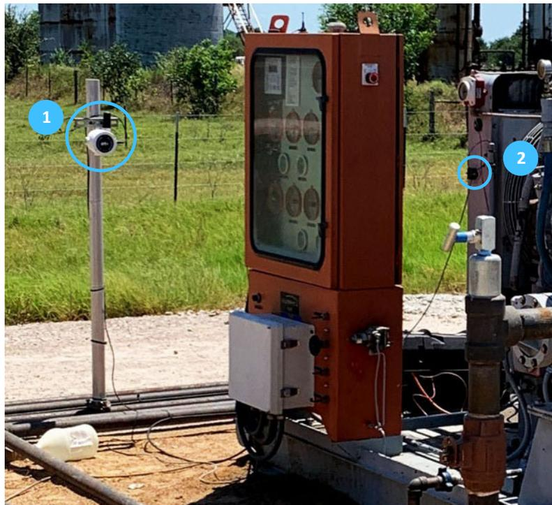
*Pictured: 1) Wireless Transmitter and 2) Vibration Sensor*
